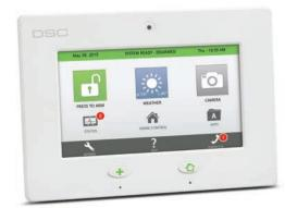
7" TouchScreen with built-in camera and compatible with DSC 433 Mhz one-way wireless products
